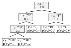
(b) Coding tree generated based on Huffman encoding.
