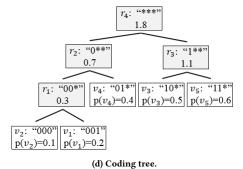
Figure 4: Sample variable-length coding scheme
